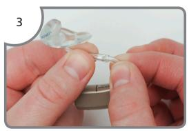
Push the tube onto the end of the hearing aid
